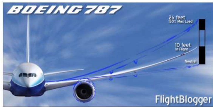
Deflection profiles of Boeing 787 for different flight loads (FlightBlogger)
